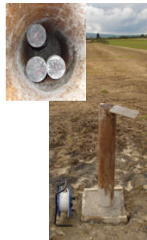
Borehole at Oakpark, Carlow. Superimposed image shows aerial view of borehole with 3 piezometers.
