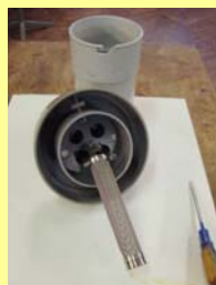
Figure 1. Photo of a passive air sampler and its shelter (behind)
